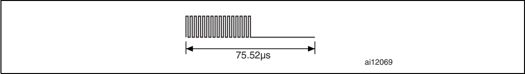
Figure 28. Logic 0, low data rate, fast commands
